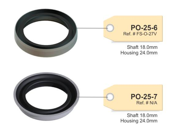
**PO-25-7** flanged metal clad seals are used in late ZF torque converters and are installed in the front cover. The OE flange design guarantees installation of the seal in one direction only and makes it impossible to make a mistake by installing it in the wrong direction.
